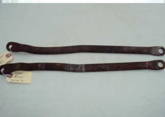
#50454 Connector/Adjustment rod connects between rail one and two. Available in passenger and drivers side. This is the rod you use to correct the sag on the sides. Order drivers or passenger side. $25.00 each
