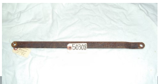
# 50308 Connects rail 3 to rail 2. Available in Drivers & Passenger. $20.00 each
