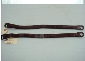
#50454 Connector/Adjustment rod connects between rail one and two. Available in passenger and drivers side. This is the rod you use to correct the sag on the sides. Order drivers or passenger side. $20.00 each
